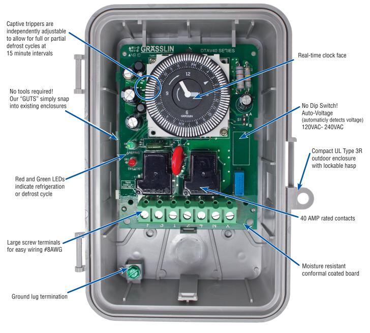
DTAV40 120-240 Volts - 40 Amps **Time Initiated** Temperature, Pressure or Time Terminated
