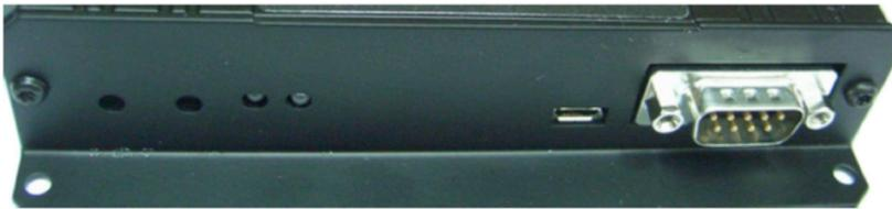
**Note:** When the Gateway is first powered, the lights 1 and 2 will turn on for a moment, turn off, and then turn back on after 30 – 60 seconds. When this cycle is complete, the buffer is connected. Light 1 will be green and Light 2 will be amber
