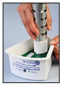
• Once housing and cell are free from mounting plate, grasp cell and turn counterclockwise while pushing down to release cell from housing.
