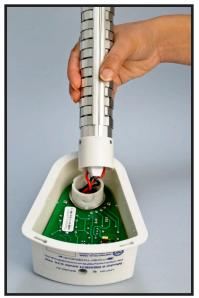
• Pull cell away from housing until lamp connector is visible.
