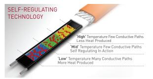
The simple 120 V Plug-n-Play system is ideal for residential and small commercial buildings and requires no specialist electrical knowledge. Simply fix to the pipe, insulate and plug into a ground-fault protected electrical outlet. It is that simple.
