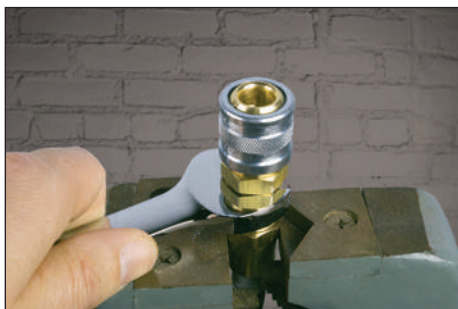
7 Tighten reusable hose barb into ferrule ensuring hose stays completely inserted.
