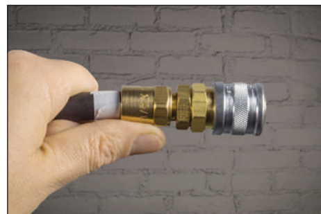
8 Completed connection, ensuring hose is completely inserted.
