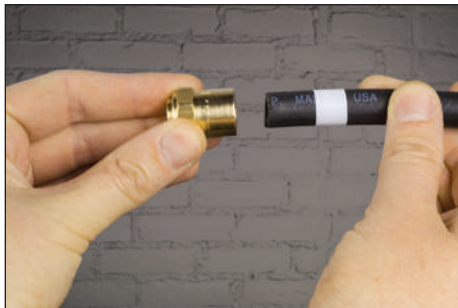
3 Mark the point of full hose insertion depth with a piece of tape.
