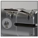
Start the crimp to the left of the duct or pipe lock-seam. With the lever in the up position, the maximum crimping depth is factory set for optimal results in 26 to 28 gauge (0.56 to 0.48 mm) galvanized steel. Back off the lever for lighter metals or re-adjust the maximum crimp, per operators manual, for heavier metals. A clutch in the gear mechanism prevents damage to the crimper attachment if seams are encountered that exceed crimper capacity.
